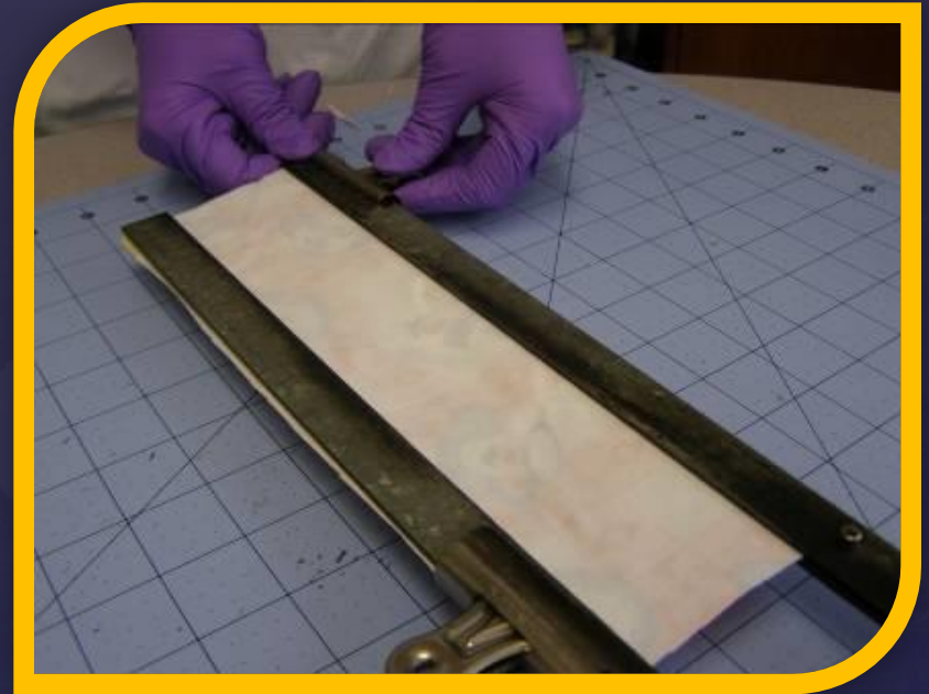
Specimen is placed in a metal holder.
